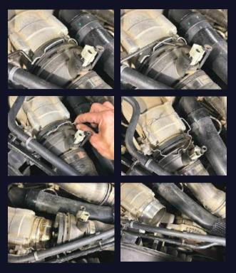
Using a pick or flat blade screwdriver remove the factory retainer clip. Slide the couplers off and remove the OEM plastic pipe.
